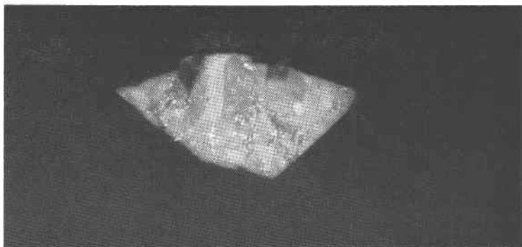
FIG. 3. Autoradiograph of polished section of euxenite, Cotopaxi, Colorado. 2X. Figs. 2 and 3 are of specimens from the same pegmatite. Note extreme variation in radioactivity of specimen of Fig. 2 and moderate variation in that of Fig. 3 but with a totally different distribution pattern.
