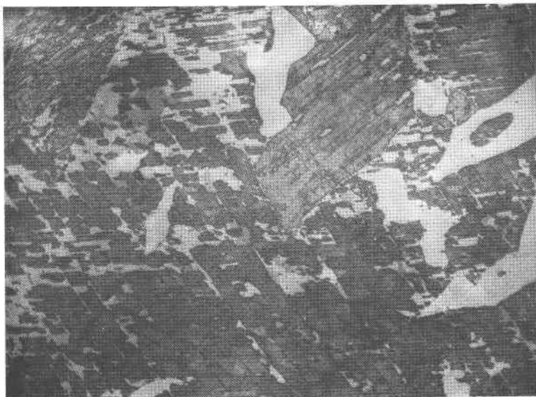
FIG. 4. Graphic to lamellae-layered texture. Dolomite grains and "veinlets" (light gray unetched) in calcite (darker gray, etched by diluted acetic acid). Chino limestone, Crestmore, California. Polished section, \times 168 .
