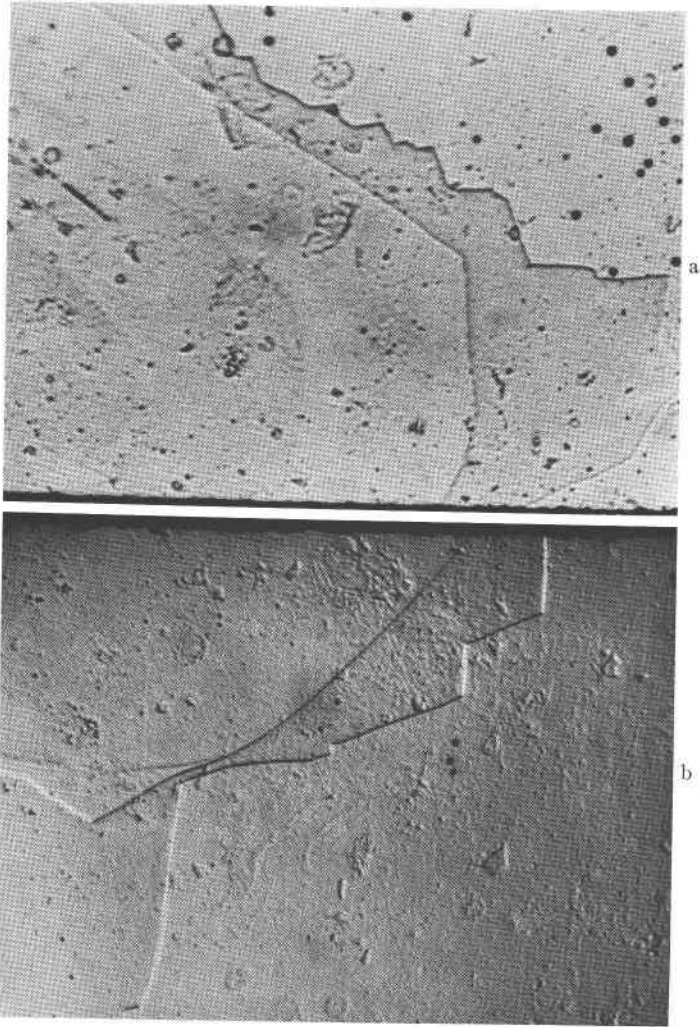
FIG. 9. Diamond no. 403 (Tanganyika, type 1). The diamond was a dodecahedron with curved faces. Two perpendicular etched sections through the same feature are shown, the one (a) being approximately (100), the other (b) being approximately (010). The common edge of the two sections which was produced by polishing appears near the lower margin of (a) and the upper margin of (b). Magnification 193\times .
