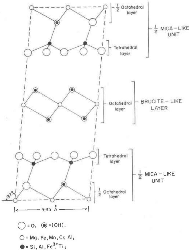
FIG. 1. Unit cell of chlorite 010 plane.
