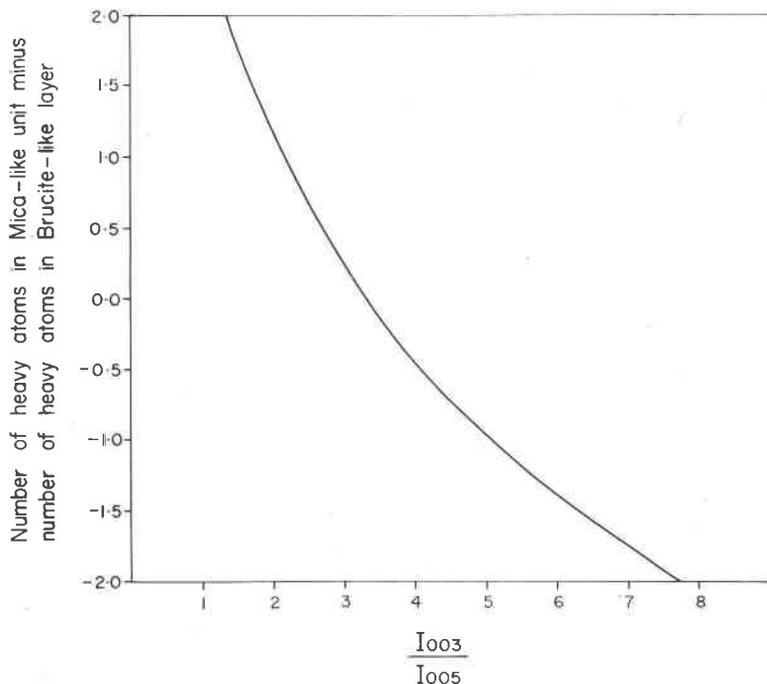
FIG. 2. Relationship between "degree of asymmetry" (number of heavy atoms in mica-like octahedral layer minus number of heavy atoms in brucite-like layer) and the ratio  $I_{003}/I_{005}$ .
