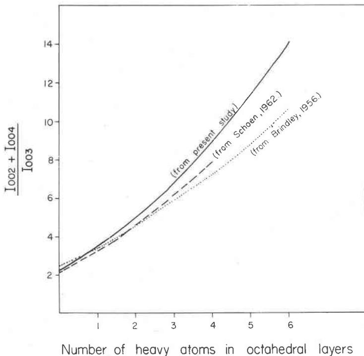
FIG. 3. Theoretical relation between number of heavy atoms in octahedral layers of chlorite and  $(I_{002} + I_{004})/I_{003}$  for  $\text{FeK}\alpha$ ,  $\text{CuK}\alpha$  and  $\text{CoK}\alpha$  radiation.
