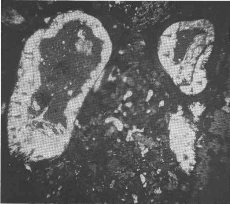
FIG. 2. Leucophosphite in cavities. Area is 1.5 mm across. The white areas are nearly pure leucophosphite. The black areas with rough or shiny surfaces are maghemite, martite, and magnetite. The dark-gray to black areas with metacolloidal structure, particularly prominent around the cavity at upper right, are mixtures of limonite, leucophosphite, strengite, and metastrengite. The gray areas in the central part of the two larger cavities are voids.
