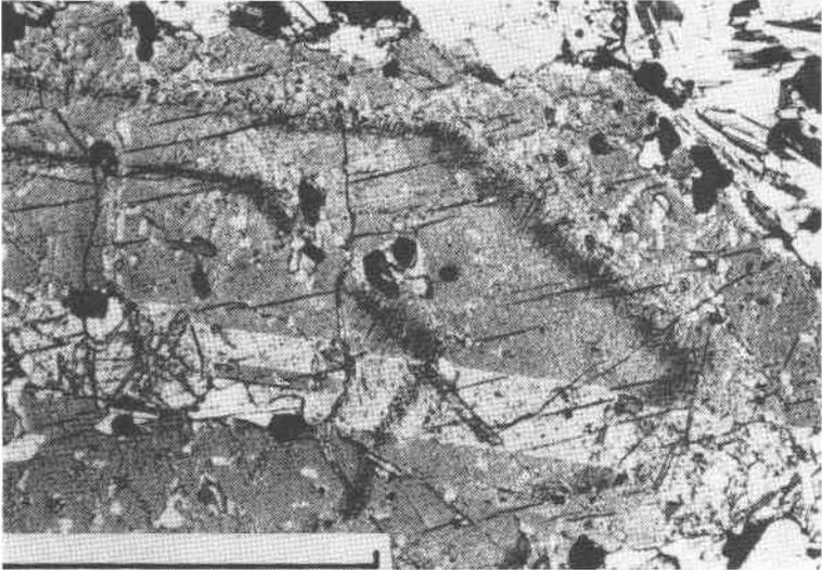
FIG. 1. Twinned pyroxene crystal showing zoning by inclusions. Note abundant plagioclase inclusions in the outer zone and the narrow bands of rutile rods in a sagenitic web. Crossed polars. Scale mark is 1 mm in length.
