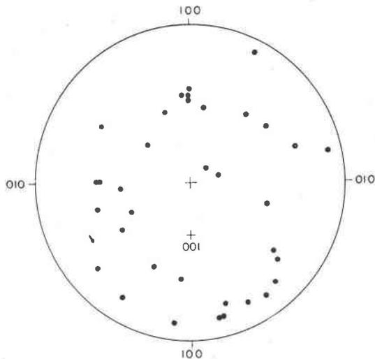
FIG. 3. Composite plot of orientation data from eighteen thin sections of graphic granite from the Ramona district showing the points of emergence of the  $c$  axis of quartz on an equal area projection of a monoclinic potassium feldspar.
