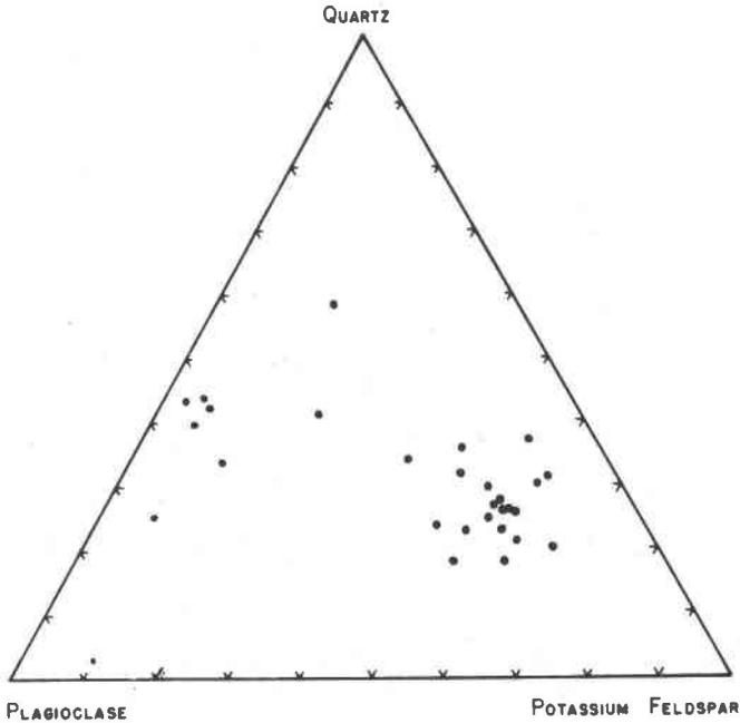
FIG. 2. Normative quartz, potassium feldspar, and plagioclase in graphic granite from other pegmatite districts. From data listed by Washington (1917), Fersman (1931) and Staatz and Trites (1955).
