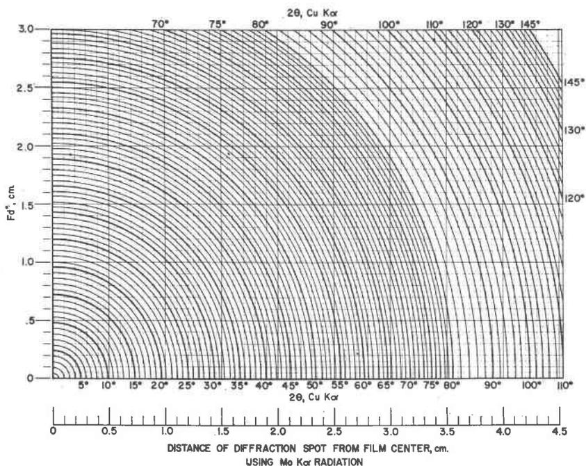
FIG. 3. Nomogram for converting precession spot distances on a precession film made with  $\text{MoK}\alpha$  into  $2\theta$   $\text{CuK}\alpha$  values.
