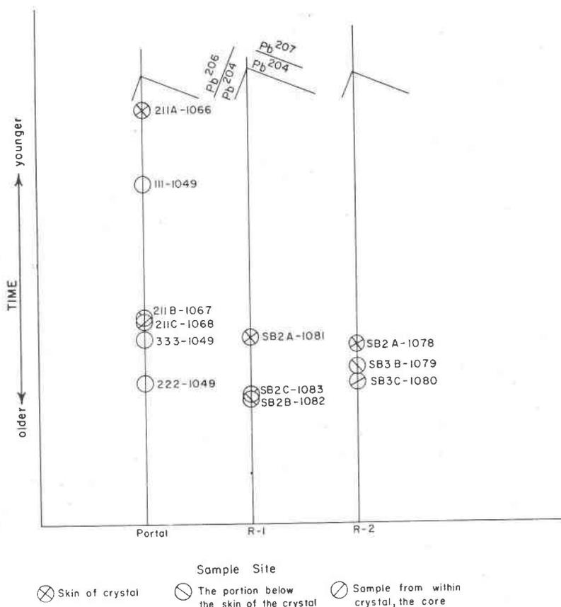
FIG. 4. Time correlation chart for various portions of three galena crystals collected in the No. 1 entry.
