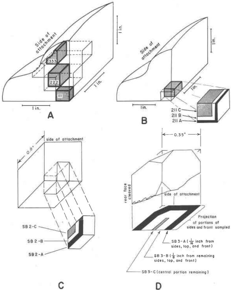
FIG. 2. Sample locations within single galena crystals. A, portal crystal, diagonal sampling; B, portal crystal, edge sampling; C, R-1 crystal; D, R-2 crystal.
