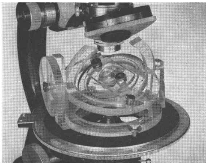
FIG. 2. The perspex stage, mounted on a Swift Model P microscope.
