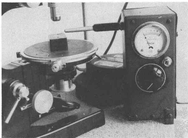
FIG. 1. The micro-coil in position for heat-etching of a polished section.
