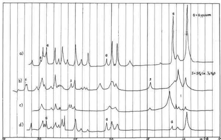
FIG. 4. X-ray diffraction goniometer traces of impure ranquillite.
