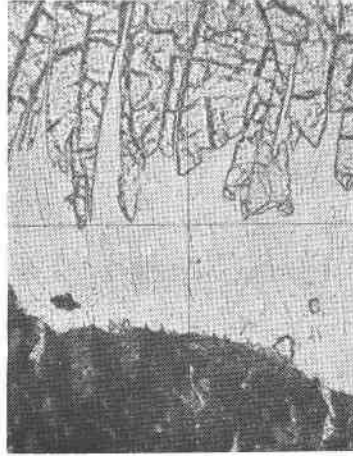
FIG. 2. Photomicrograph showing banded structure in antigorite. Crossed nicols. \times 40 .
