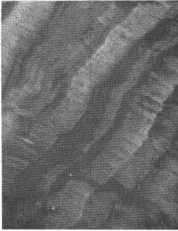
FIG. 2. Photomicrograph showing banded structure in antigorite. Crossed nicols. \times 40 .
