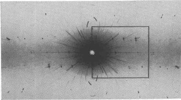
FIG. 2. Oscillation photograph about  $z$ -axis of an augite crystal containing pigeonite lamellae, taken with filtered Fe radiation. At the centre of the oscillation range the  $x$ -ray beam was parallel to the diad  $y$ -axis. The black lines indicate approximately the region illustrated for different specimens in Figs. 3 to 8. With the exception of Fig. 4, all diffraction patterns were obtained with filtered Fe radiation. [Specimen from Mt. Wellington, Tasmania.]
