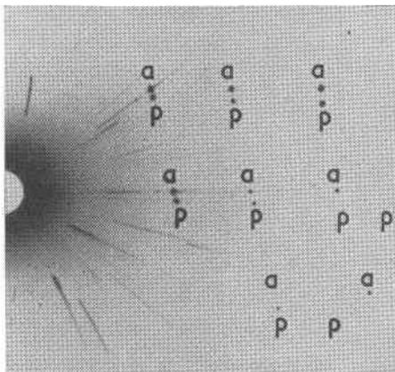
FIG. 3. Augite (*a*), with exsolved pigeonite (*p*). [Specimen from Skaergaard Intrusion, E. Greenland. No. 1691.]
