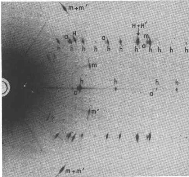
FIG. 7. Initially single-phase volcanic hypersthene (*h*), which on being heated at 1050° C. in air has exsolved "twinned" augite (*a*, *a'*), magnetite (*m*, *m'*) and haematite (*H*, *H'*). The origin of the short streaks marked ? is uncertain: they may be from an oriented form of silica. [Specimen from Koolau, Oahu.]
