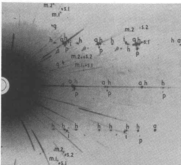
FIG. 6. Augite (*a*), with both pigeonite (*p*) and hypersthene (*h*). Other phases are ilmenite (*i*), magnetite and spinel (probably hercynite) each in two orientations (*m.1*, *m.2*, *s.1*, *s.2*). *g* indicates spots from a disoriented fragment, and  $\beta$  those produced by  $\text{FeK}\beta$  radiation. (A few spots due to clino-amphibole are also present but are unmarked.) [Specimen from Kragerø, Norway.]
