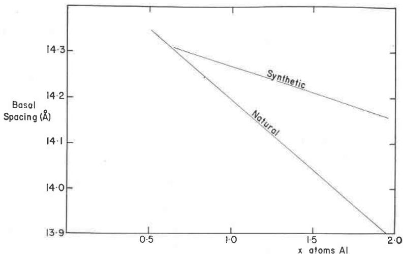
FIG. 2. The variation of the basal spacing of chlorites with composition. (The curve for the natural chlorites is taken from Brindley and Gillery, 1956.)
