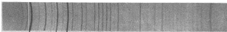
FIG. 1. X-ray powder photograph of genthelvite from Jos, Northern Nigeria. The three strongest lines are 3.33Å, 2.174Å and 1.918Å. CuK radiation, Camera diameter 9 cm.
