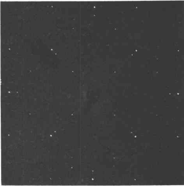
FIG. 1. Gillespite: hk0 precession pattern. Unfiltered Cu radiation. Exposure 4 hours.
