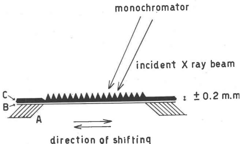
FIG. 1. Design of the sample holder (A), with cellophane (B) and the rippled clay surface (C).
