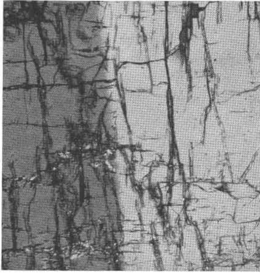
PLATE 2. Zoned andalusite showing \{110\} cleavage and parting parallel to \{001\} . Section \perp a with X approximately N.S. Note minor development of fine-grained muscovite (bright material) along cleavage and parting cracks, but absence of corundum. Crossed nicols with analyzer 45^\circ from X, \times 27 .
