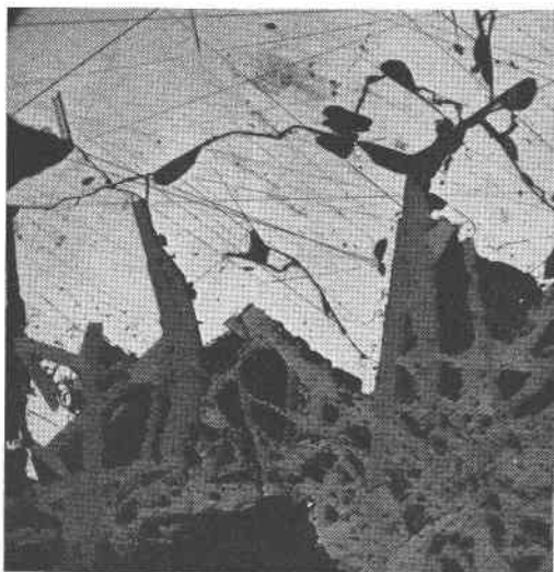
FIG. 1. Boxwork of nolanite (gray) in chalcopyrite (white) and dolomite (black). Polished section of weathered specimen, Zone "A," Eldorado Mining and Refining Ltd., Fish Hook Bay. Magnification 100 \times .
