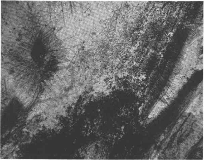
FIG. 5. Intense alteration of muscovite to diaspore and boehmite around an etch pit (upper left) and a shear plane (lower right). In the lower half of the photograph much of the muscovite surface is covered by a dark deposit of boehmite, diaspore, hematite, and the spinel-group mineral. In plane-polarized light, \times 53 .
