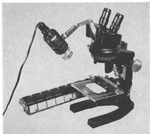
FIG. 1. Equipment used for modal analyses on rock slabs.
