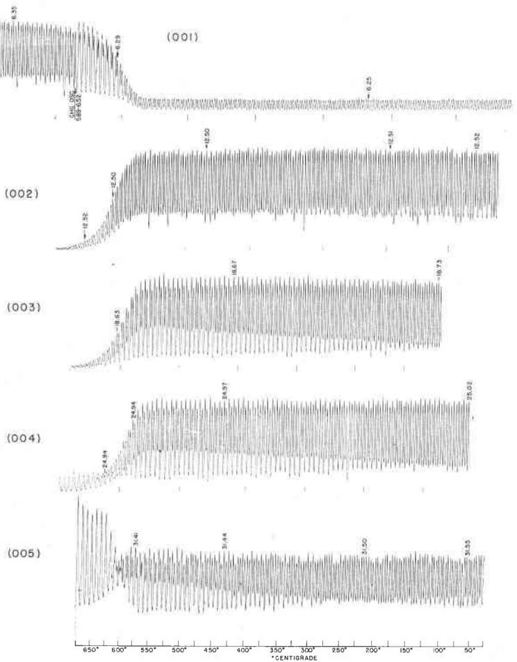
Fig. 4. Heating-oscillating patterns of five orders of the basal spacing of clinocllore.
