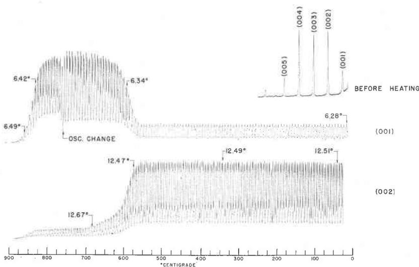
FIG. 3. Heating-oscillating patterns of two orders of the basal spacing of sheridanite.
