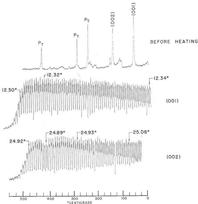
FIG. 2. Heating-oscillating patterns of the first and second order of the basal spacing of kaolinite.
