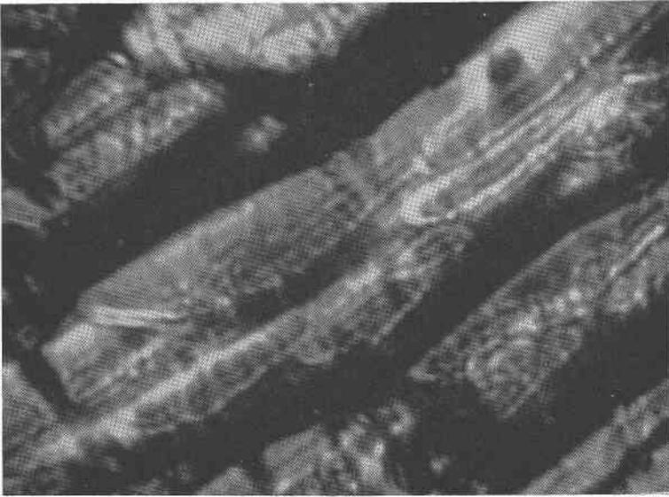
FIG. 2. An enlargement (200 $\times$ ) of the same area shown in Fig. 1. Here the regularity of the layers and the individual rods can be clearly seen. An isolated rod in a layer can be seen in the upper left part of the photomicrograph.
