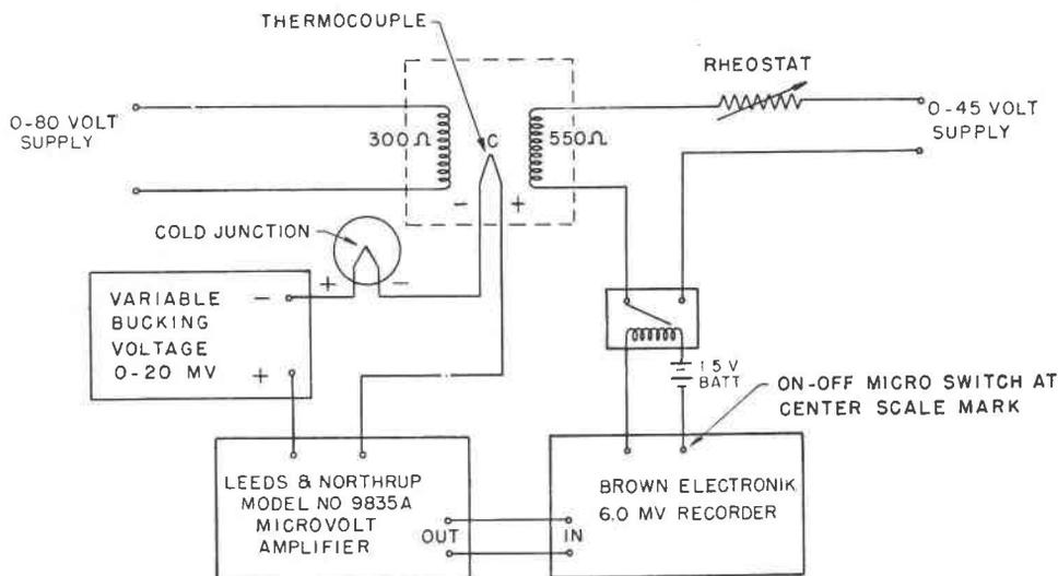
FIG. 3. Block wiring diagram of heater control circuits.
