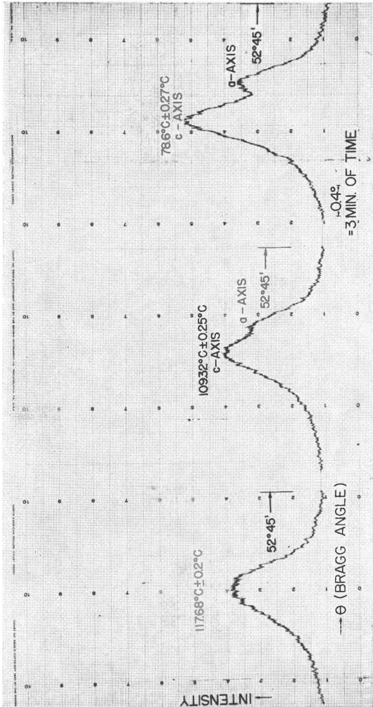
FIG. 4. X-ray intensities as a function of angle for single crystal oven. The 4th order reflection of BaTiO<sub>3</sub> tetragonal to cubic phase change for Cu K radiation is used to check the crystal vs. thermocouple temperature.
