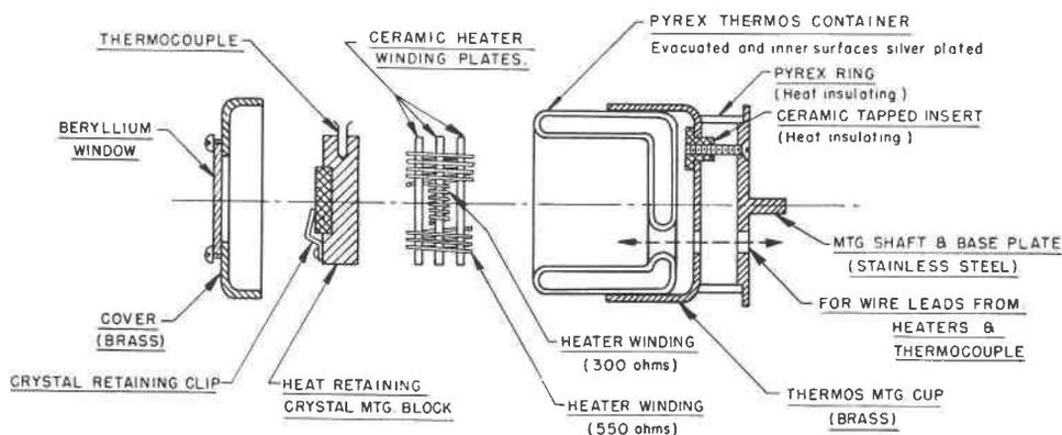
FIG. 1. Exploded cross-sectional view of heater.
