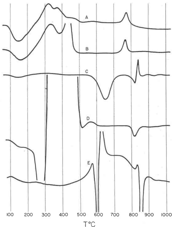
FIG. 1. Differential thermal analysis patterns of (A) ekmanite, (B) stilpnomelane, (C) clinocllore, (D) ferrous oxalate and (E) sodium oxalate.
