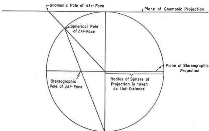
FIG. 2. Construction of the gnomonic pole of a face from its stereographic pole in the case of a triclinic crystal.
