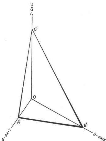
FIG. 7. Relationship of the unit plane 111 to the unit distances along the  $a$ -axis,  $b$ -axis, and  $c$ -axis in the case of a triclinic crystal.
