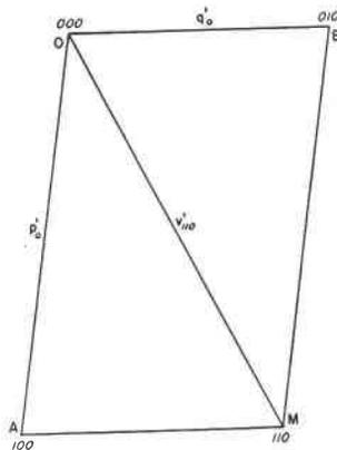
FIG. 4. Relationship of the polar lattice elements  $p_0'$  and  $q_0'$  of a triclinic crystal to the interfacial angles  $100 \wedge 110$  and  $010 \wedge 110$ .
