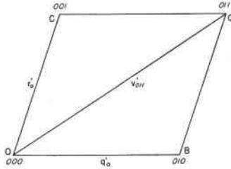
FIG. 5. Relationship of the polar lattice elements  $q_0'$  and  $r_0'$  of a triclinic crystal to the interfacial angles  $010 \wedge 011$  and  $001 \wedge 011$ .
