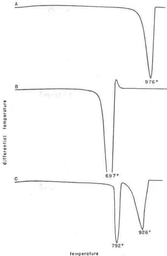
FIG. 8. Differential thermal analysis curves. *A*, calcite no. 13, Joplin, Missouri, record *C-89*, resistance in series with the galvanometer 999.9 ohms. *B*, Magnesite no. 1, Windous deposit, White Pine County, Nevada, record *C-79*, resistance in series with the galvanometer 999.9 ohms. *C*, Dolomite, Millville, West Virginia, Record *F-3*, resistance in series with the galvanometer 900 ohms.
