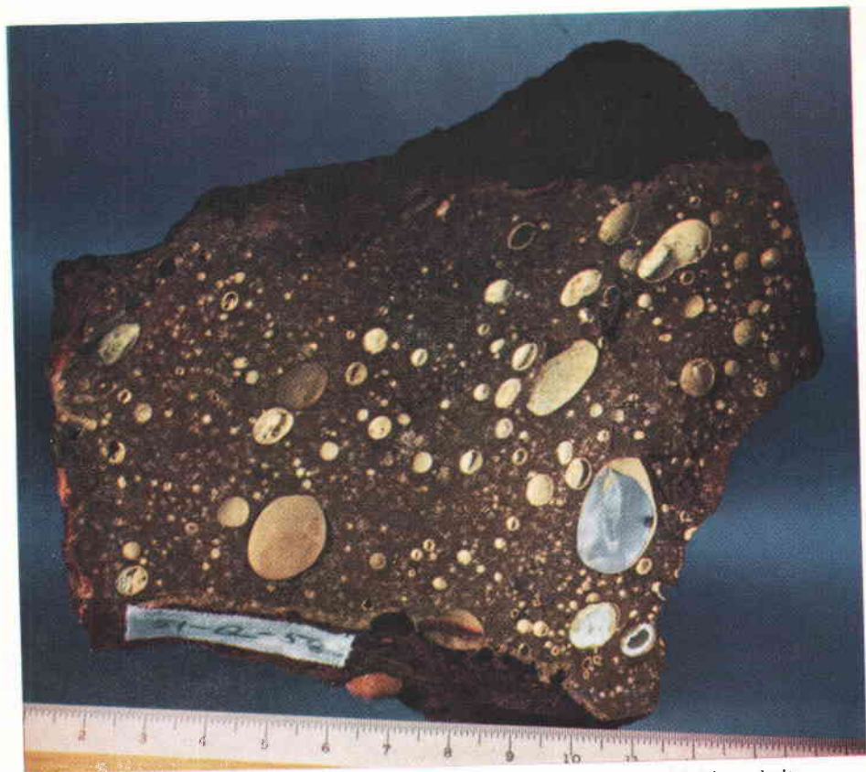
PLATE I A. Color photo showing manner of occurrence of the amygdules in andesite. Scale is in centimeters.
