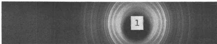
FIG. 1. X-ray powder contact print of cuprobismuthite from Park county, Colorado. Nickel filtered copper radiation; 1^\circ\theta=1 mm.
