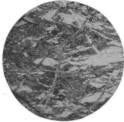
FIG. 5. Protomylonite. Red feldspar porphyroblast 0.7 mm. wide in fine flow-textured groundmass of quartz and muscovite.
