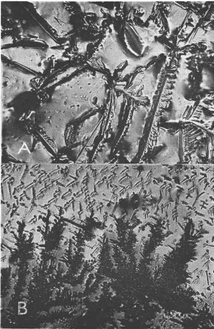
FIG. 2. Fractographs of cast molybdenum metal illustrating Type Ic patterns for heterogeneous constitution. (Above) Featherlike intergranular structures expressing carbide. 440 \times . (Below) Dendritic growths of intergranular oxide encroaching upon featherlike carbides as shown above. 320 \times .
