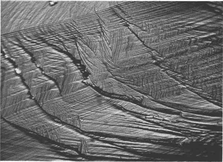
FIG. 11. Fractograph of twinned calcite. 235 \times .
