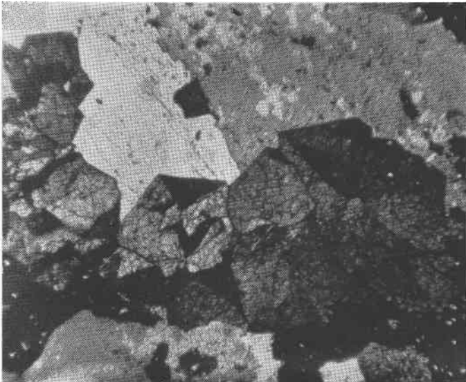
FIG. 4. This section \times 100 , crossed nicols. Andradite garnet and natrolite. Shows birefracting segments in andradite.
