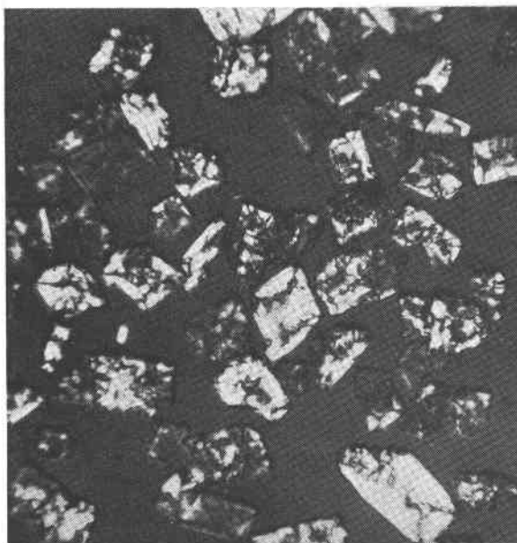
FIG. 3. Optically anomalous periclase resulting from the conversion of magnesite grains (-150+200 mesh) to the oxide by heating. Crossed nicols. Mag. about 75X.
