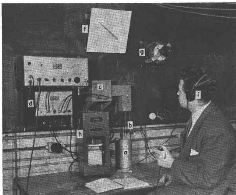
FIG. 2. Photograph of the apparatus in use. (a) Small electric muffle furnace, (b) glass tube carrying the charge, (c) microphone in sound insulating box, (d) audio amplifier, (e) electronic relay, integrating circuit, and power amplifier (f) temperature indicator, (g) variable transformer for controlling the furnace, (h) recording millimeter, (i) monitoring ear-phones, (j) push switch for producing temperature fiducials on the curve.
