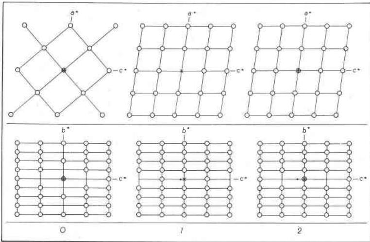
FIG. 11. 0, 1, 2 levels reciprocal lattice nets shown by (upper row)  $b$  and (lower row)  $a$  axis precession photographs of lindgrenite.
