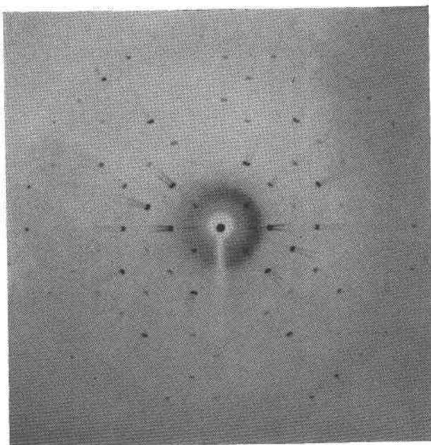
FIG. 4. Lindgrenite,  $b$  axis, first level (Mo) ( $c^*$  horizontal)
