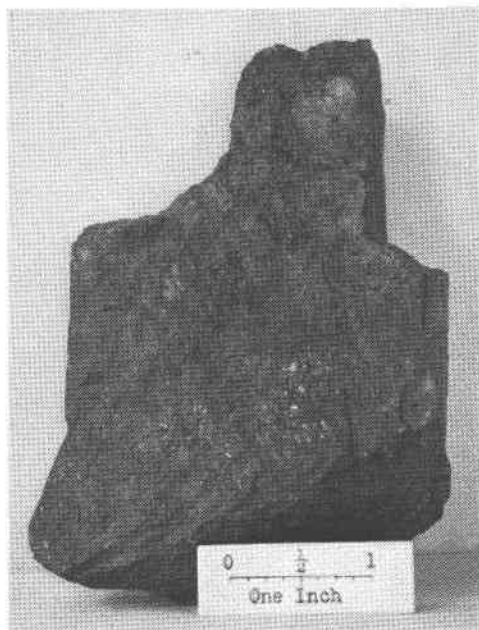
FIG. 3. Photograph of largest monazite fragment found in Yard pegmatite. The shiny spangles are specular hematite.
