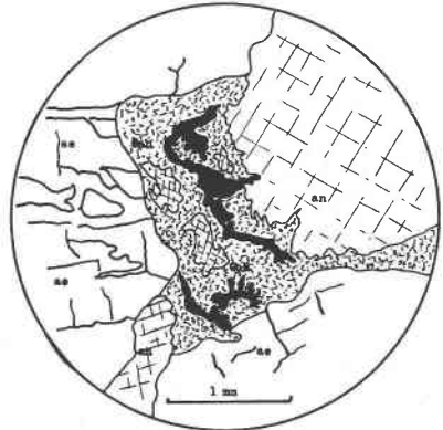
FIG. 2. Drawing of thin section from the 2113 level in the footwall ore zone, showing magnetite (black) in the crushed anhydrite (can) zone as well as a tongue into the anhydrite (an) crystal. Aegirinaugite (ae)
