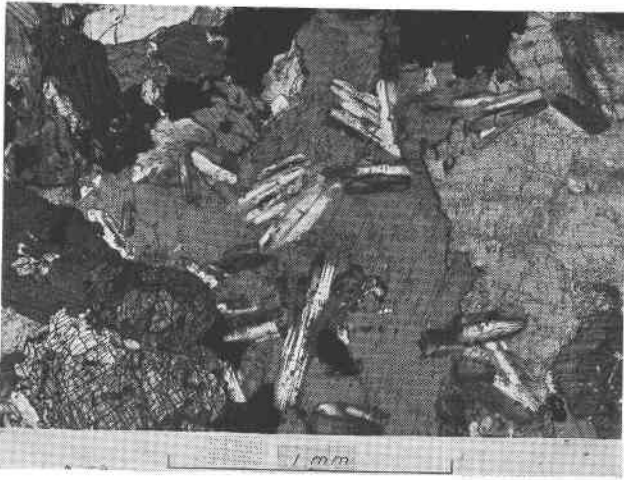
FIG. 3. Photomicrograph of a thin section of monzonite (crossed nicols).
