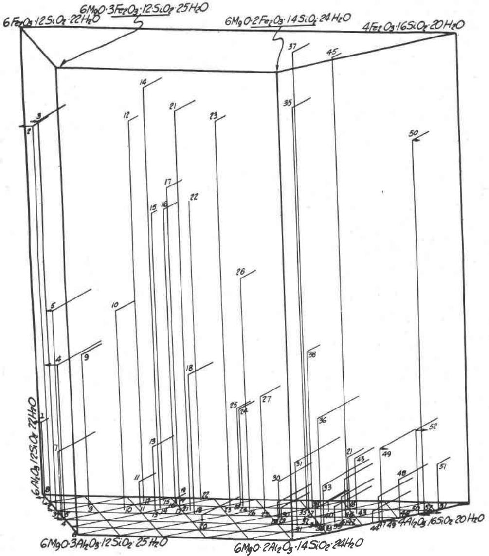
FIG. 2. Montmorillonite analyses in a three-dimensional figure whose base is shown in Fig. 1.
