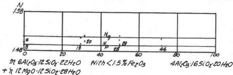
FIG. 3. Indices of refraction of montmorillonites (containing less than 1.5% Fe<sub>2</sub>O<sub>3</sub>) with varying replacement of Si by Al.
