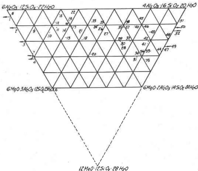
FIG. 1. Montmorillonite analyses plotted on (part of) a triangle having  $4\text{Al}_2\text{O}_3 \cdot 16\text{SiO}_2 \cdot 20\text{H}_2\text{O}$ ,  $6\text{Al}_2\text{O}_3 \cdot 12\text{SiO}_2 \cdot 22\text{H}_2\text{O}$ , and  $12\text{MgO} \cdot 12\text{SiO}_2 \cdot 28\text{H}_2\text{O}$  at its corners, Al standing for Al, Fe''', Ti and Cr, and Mg for Mg, Fe'', Mn, Ca.
