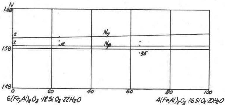
FIG. 4. Indices of refraction of montmorillonites (or nontronites) with much Fe<sub>2</sub>O<sub>3</sub> (between 10 and 13% atomic Al).
