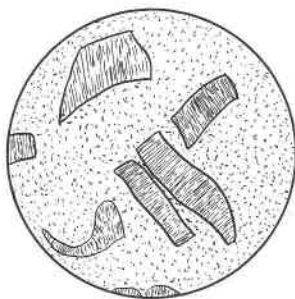
FIG. 3. Kaolinite crystals, showing perfect cleavage. Magnification 175 diameters.
