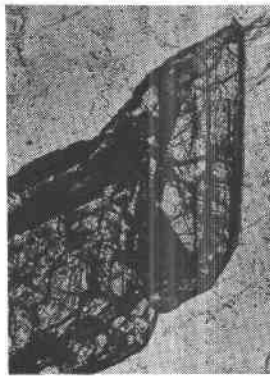
FIG. 6. Section of pumpellyite parallel to (010) in quartz matrix. Note crystal outlines and semi-opaque alteration product. \times 56 .
