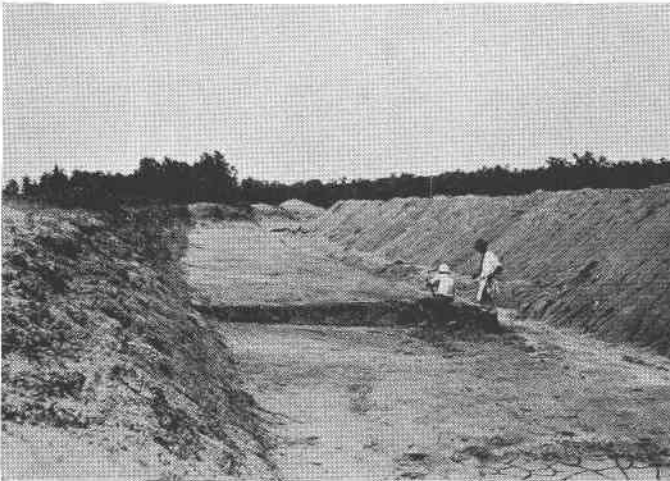
FIG. 14. Photograph of upper clay bed stripped for mining.
