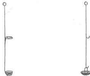
FIG. 2. Double weighing pan for single fragments.
