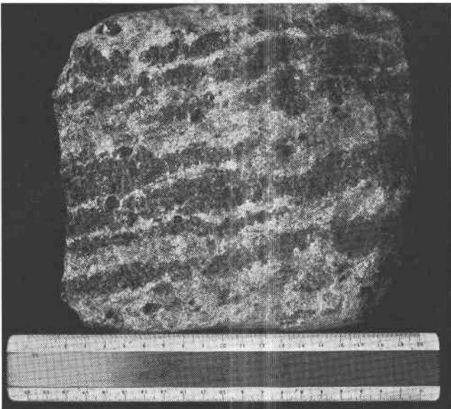
FIG. 4. Specimen of ore taken from the face shown in Fig. 3. The light bands are apatite, the dark bands nepheline.
