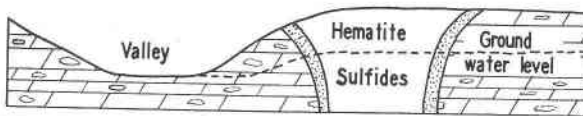
The hematite was formed from the sulfides after the water level was lowered by the downward cutting of the valley.
