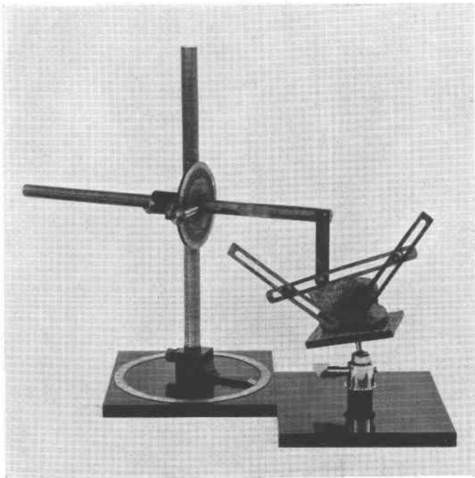
FIG. 4—Measuring and marking the plane of a thin section. The apparatus has been turned 180^\circ from its position in Figs. 2 and 3 in order to show the marking arms to better advantage. Plane of thin section, N 67^\circ W 89^\circ NE .
