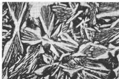
FIG. 2. The regenerated amphibole showing skeleton-growth. \times 65 .
