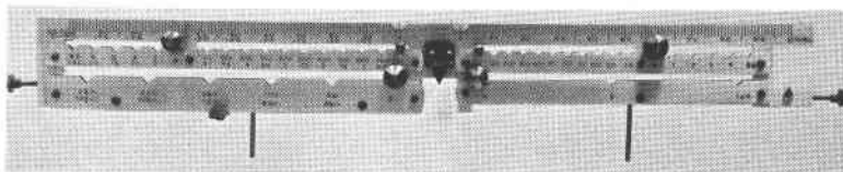
FIG. 1. The balance beam showing the arrangement of the notches and riders adopted in order to avoid the use of loose weights in specific gravity weighings.
