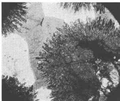
FIG. 5. Fringes of piedmontite on inclusions in quartz veins. Nicols partially crossed. Only a portion of the inclusion can be seen at the lower right. See Figs. 11 and 12 for better display of inclusions and piedmontite fringes. \times 25 .
