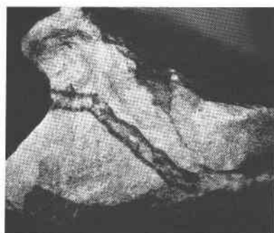
FIG. 8. A similar veinlet of piedmontite and quartz in sandstone still showing the dark borders of piedmontite. \times 1.0 .
